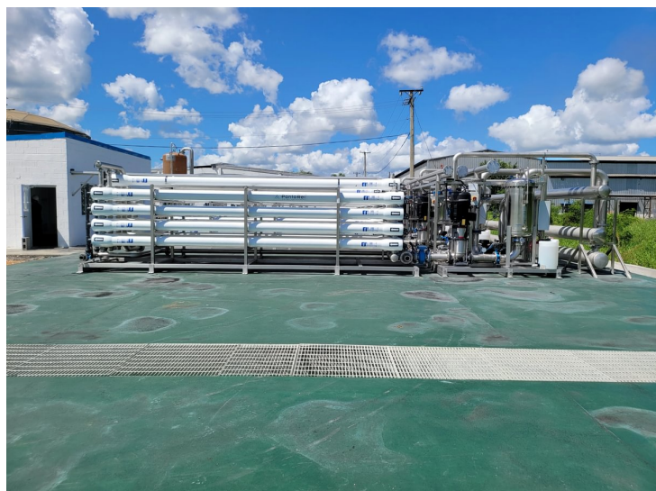
Water filtration equipment ready to ship to Bangladesh for Primark's innovative wastewater recycling and micro pollution removal project
