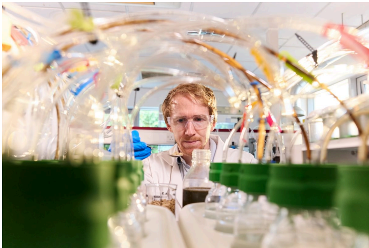
Testing the gas-yield potential of waste for use as anaerobic digestion feedstock at Amur Energy's lab in York, UK
